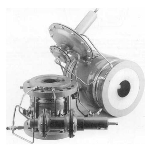
The Inbal variable pressure reducing valve, model XXX-VR, automatically reduces an upstream pressure to a lower downstream pressure which varies in a predetermined relationship, with the flow rate through the valve. At a given flow rate the downstream pressure remains stable and unaffected by fluctuations in the inlet pressure.
